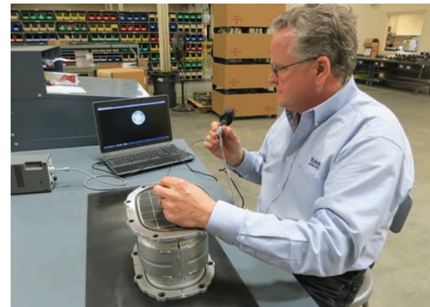
Kubota Diesel Particulate Filters are thoroughly inspected, reconditioned, painted and certified ready for service right out of the box.
